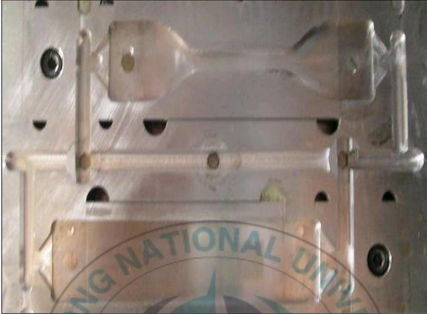
Fig. 4-2 Experimental mold with 2 cavities
