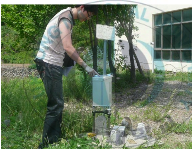
Fig. 3.3 Relative gravity measurement using CG-5 in a benchmark
