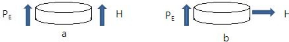
Fig.34. cylinder ceramics. (a) Poling longitudinal to the  $H_{dc}$  and  $H_{ac}$ . (b) Poling transverse to  $H_{dc}$  and  $H_{ac}$ .
