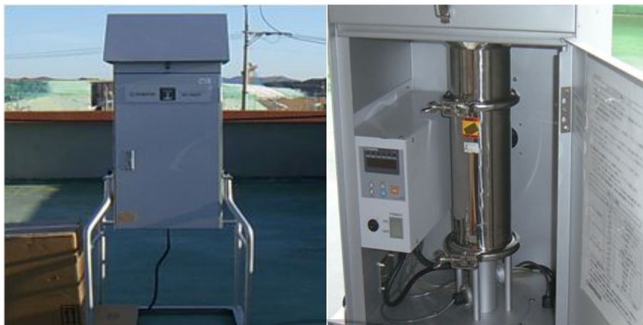
Fig. 5. High Volume Air Sampler for particulate and gas compounds.
