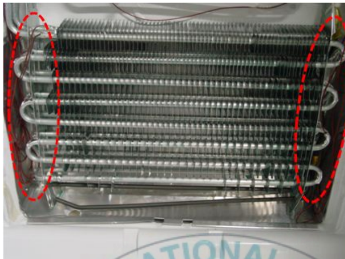
( a ) The measurement positions of temperature on evaporator
