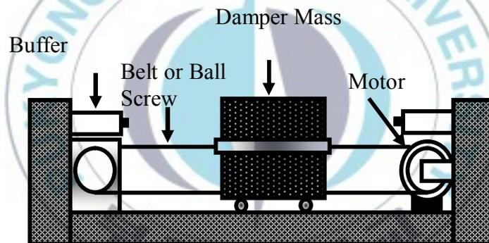
Fig. 2.2: Auxiliary mass damper
