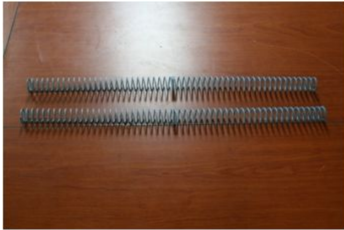
Fig. 4.1 Protection spring of water level gauge.
