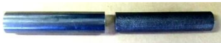
(b) Friction welding test specimens
