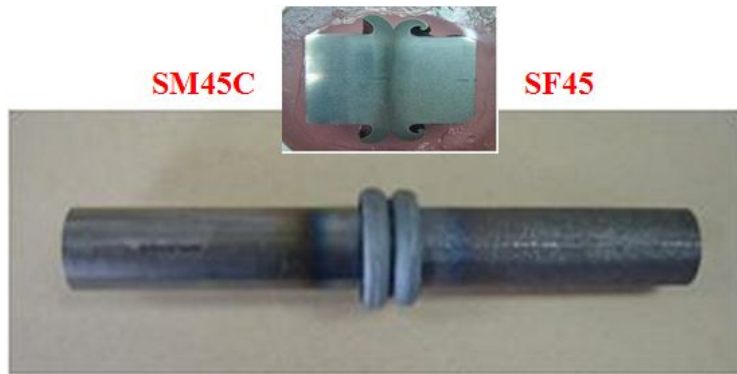
Fig. 4-3 Shape of the friction welded flash
