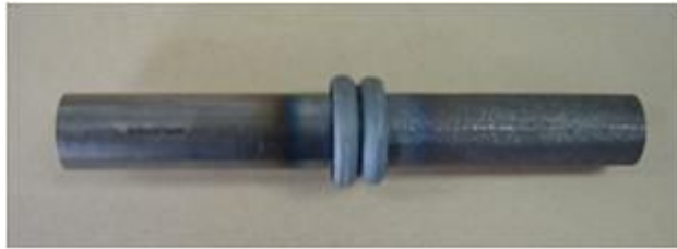
(c) Finish shape of friction welding
