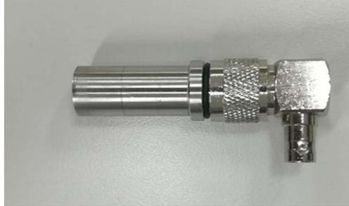
Figure 4 50 MHz Immersion Transducer
