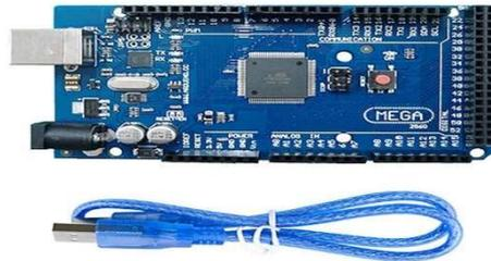
Figure 11 ATmega2560 Board<sup>8</sup>
