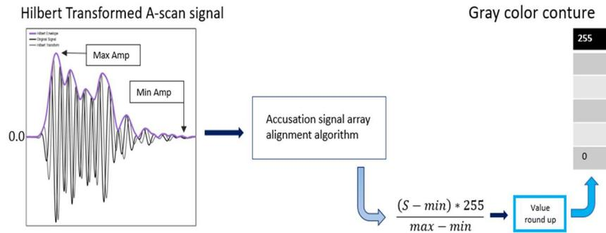
Figure 16 Acoustic signal to image formation
