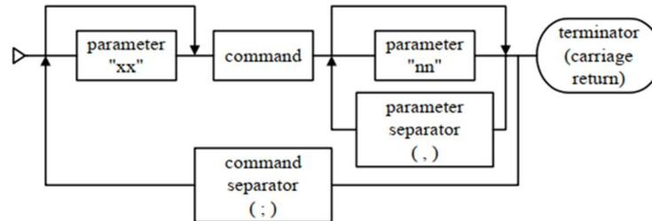
Figure 8 Command Syntax of ESP 300 Motion Controller<sup>6</sup>
