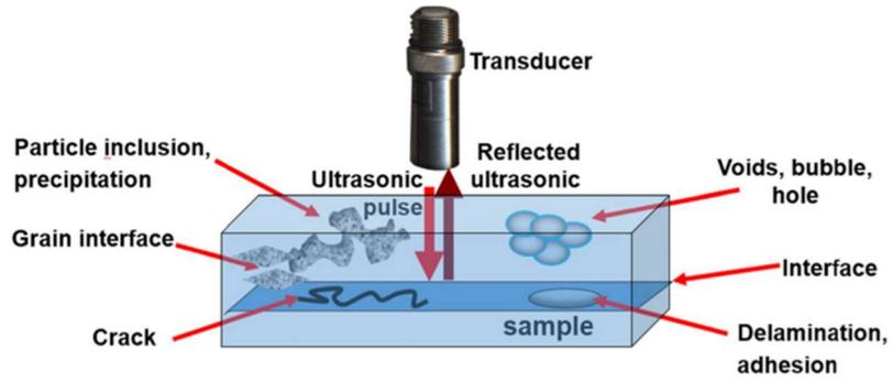
Figure 2 Transducer Pulsing and echoing from sample with numerous defects<sup>1</sup>
