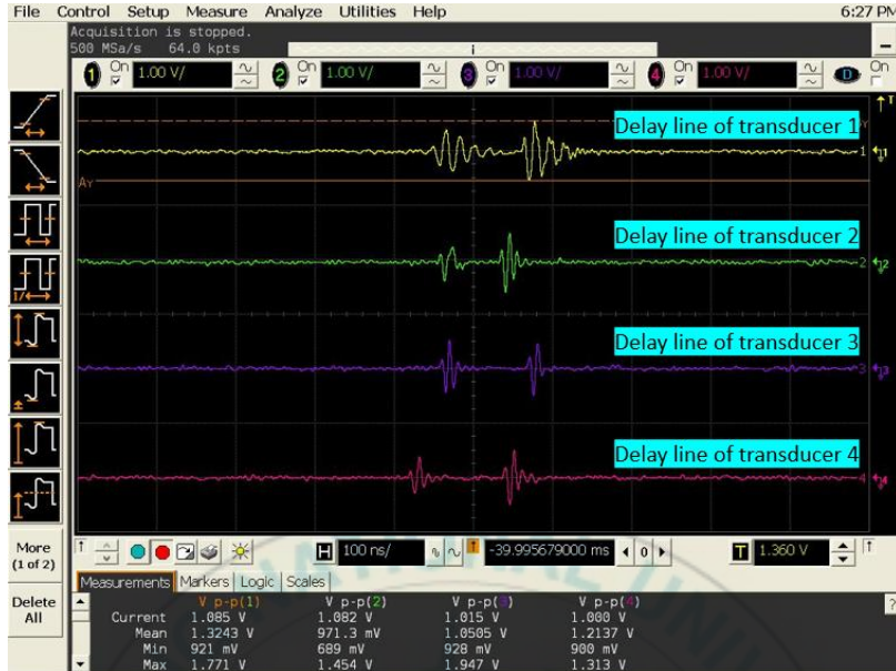
Figure 27: The signal amplitude after adjusting gain on each channel.
