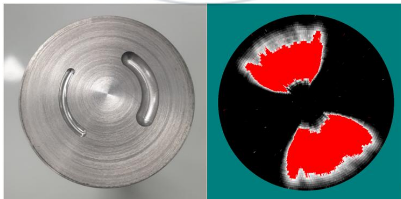
Figure 34: The acoustic imaging result of metal bar
