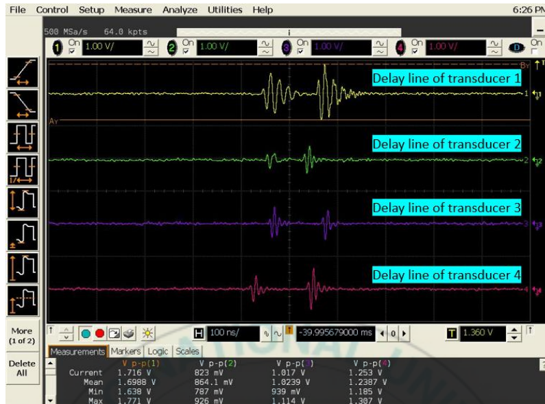
Figure 26: The different signal amplitude from 4 focused transducers
