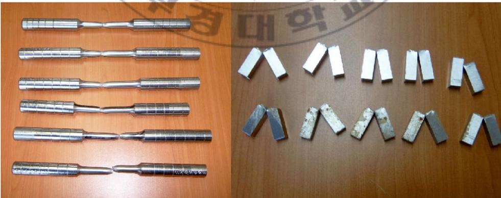
Fig. 3.15 Specimens after tensile (left) and impact (right) test
