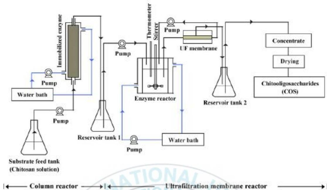
**Figure 14:** Schematic diagram of the dual reactor system developed for continuous production of chitooligosaccharide (COS). Adapted from Jeon and Kim (2000)
