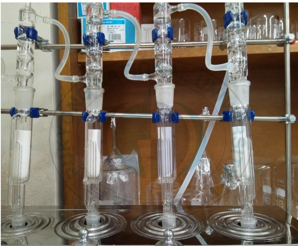
**Fig.5:** Soxhlet extraction system
