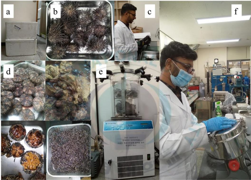
**Fig. 4:** Sample preparation process. (a) imported sample, (b) thawed sample, (c) dissection of the samples, (d) separation of the body parts, (e) freeze drying of the samples, (f) grinding the dried samples into powder.
