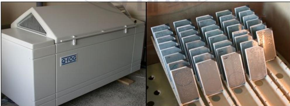
Fig. 15. Prohesion Test Equipment.
