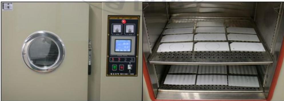
Fig. 16. Temperature & Humidity Chamber for Hygrothermal Stress.
