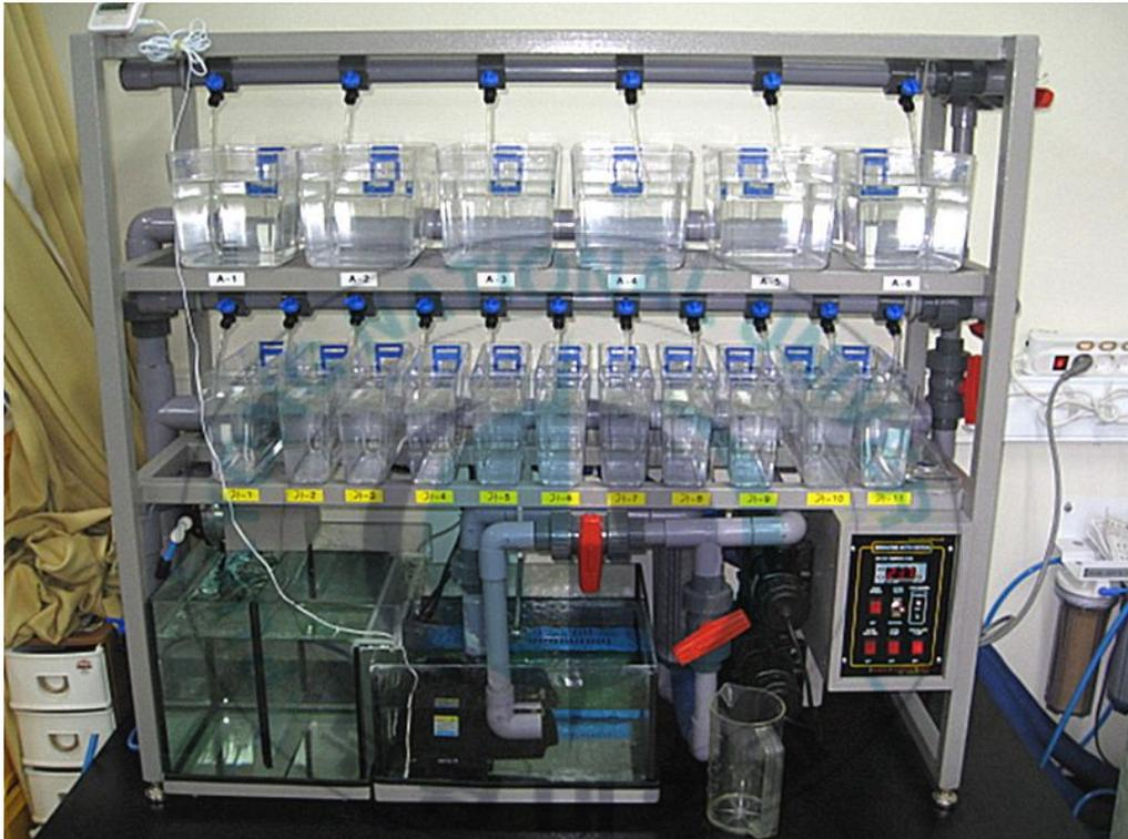
Fig. 2. Culture system for low temperature tolerance experiment.
