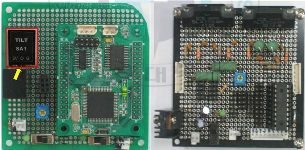
Fig. 6. 6 Two Wheel Robot's Controller and Step Motor Drive
