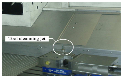
Photo. 3-3 Tool cleaning jet
