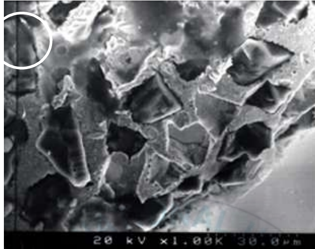
(a) Side view of grinding wheel surface
