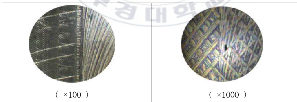
Fig. 5-28 Specimen surface after high speed grinding (depth of cut : 1\mu\text{m} , rpm : 40,000)
