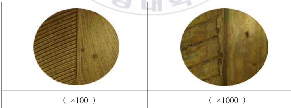
Fig. 5-20 Specimen surface after high speed cutting (depth of cut : 2\mu\text{m} )
