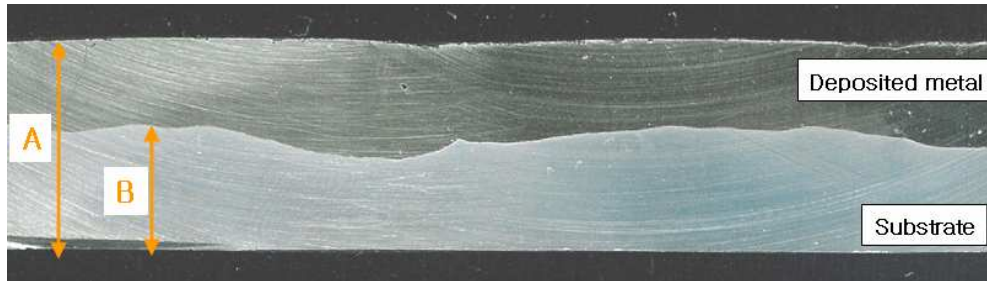
Fig. 2.2 Cross section of weld area
