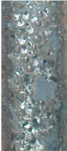
Fig. 5.1 Water glass ball on the bead surface
