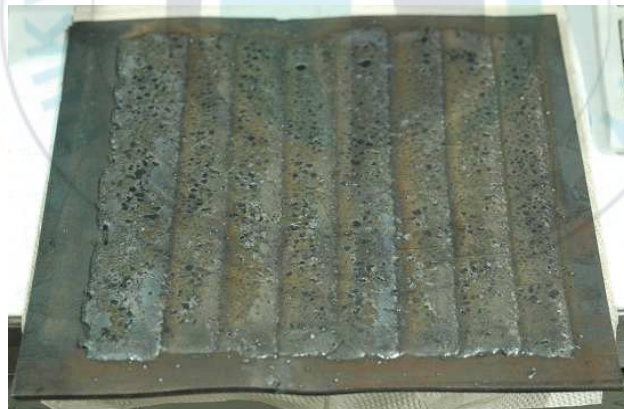
Fig. 6.5 Configuration of weld bead with Overlap
