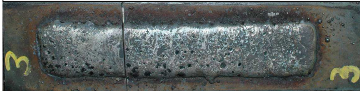
Fig. 5.5 Weld bead of CFP GMAW
