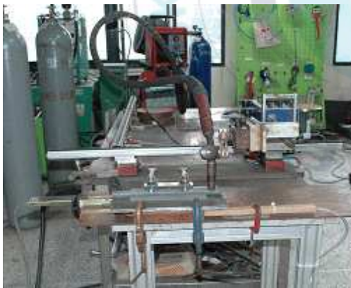
(a) Fit up of welding equipment
