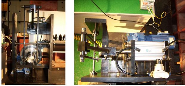
(b) Ratch and motor in test bed
