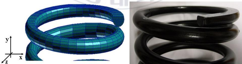
Fig. 4.3 Part of FEM model of spring.
