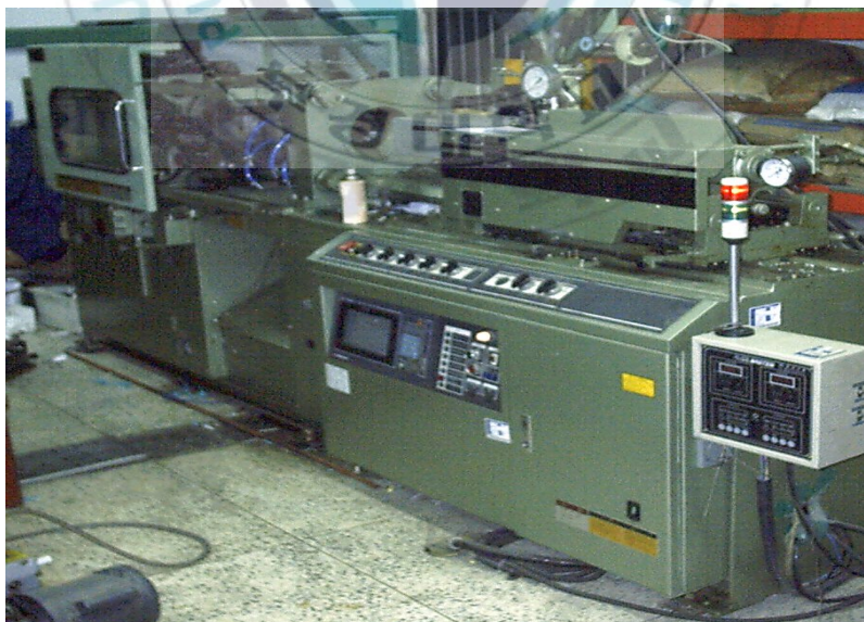
Fig. 3-1 Injection molding machine for experiment (75ton)
