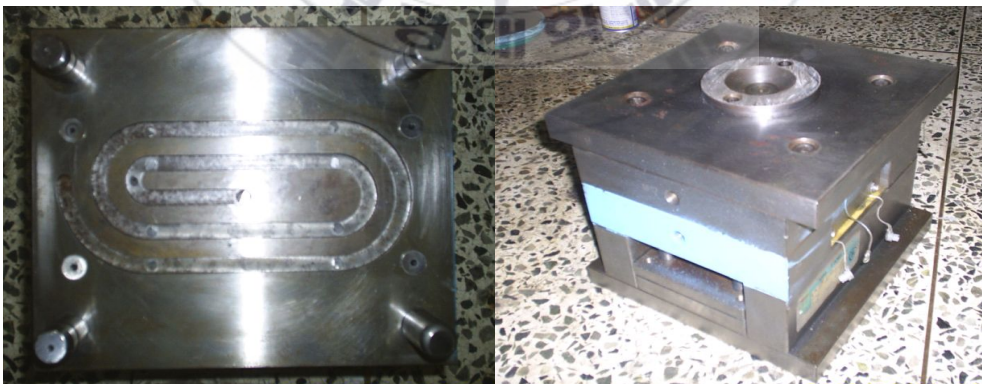
Fig. 3-5 Photo. of experimental mold (spiral)
