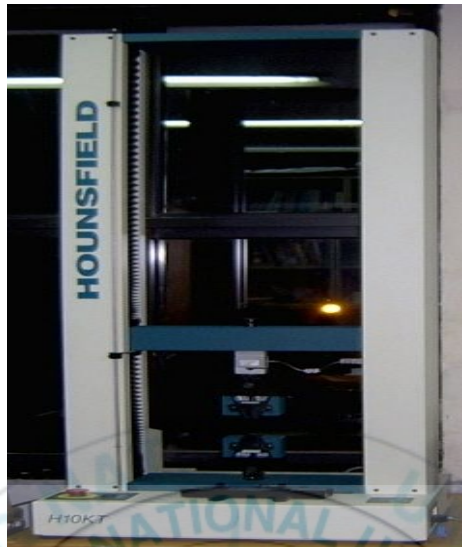
Fig. 3-7 Photo. of universal testing machine
