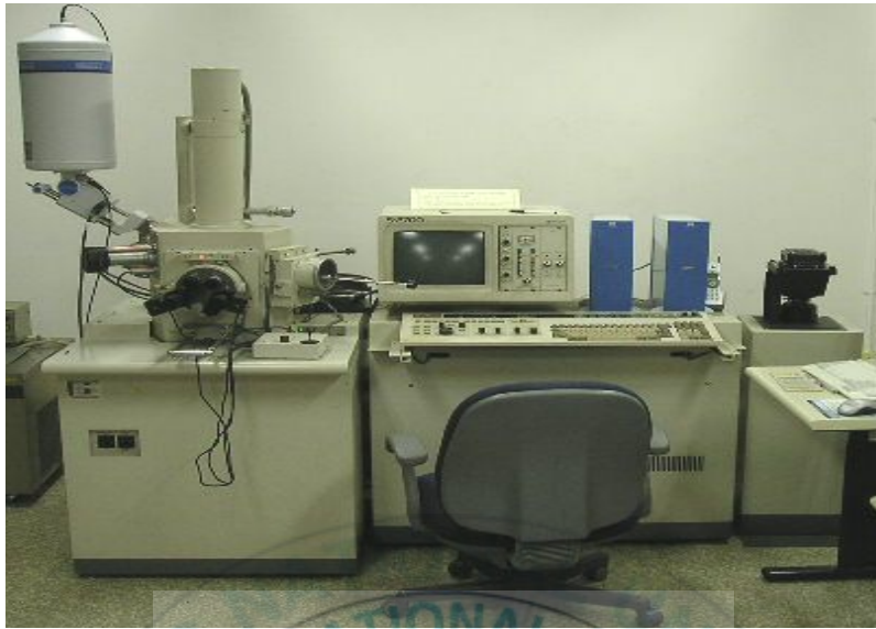
Fig. 3-11 Photo. of scanning electron microscopy
