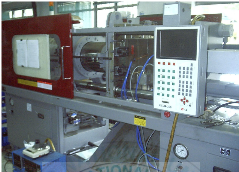
Fig. 3-2 Injection molding machine for experiment (140ton)
