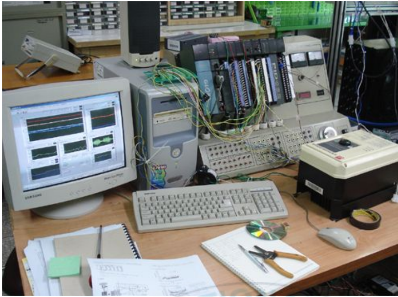
Photo. 1 Data acquisition and control system(PLC and Inverter)
