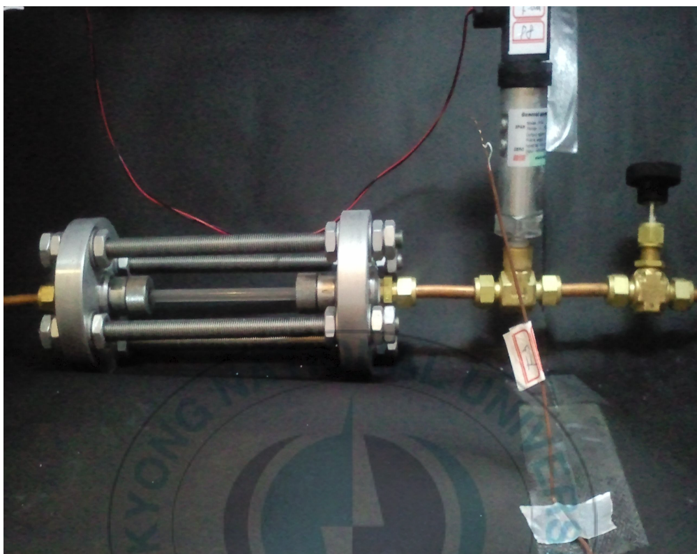
Fig.3.13 Installation of visualization equipment in F-evaporator outlet
