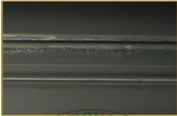
Fig.4.23 Visualization of two-phase flow in evaporator outlet (off time)
