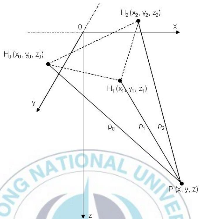
Fig. 4. 3-D coordinates of the acoustic transmitter and the hydrophone.  $\rho_0$ ,  $\rho_1$  and  $\rho_2$  are distances between the acoustic transmitter (P) and each hydrophone ( $H_0$ ,  $H_1$ , and  $H_2$ ).
