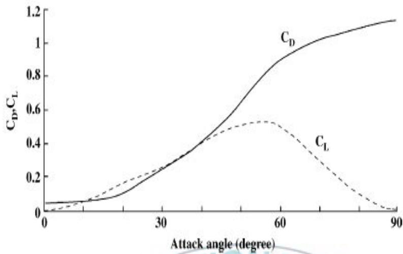
Fig. 3. The drag and sheering force coefficients for a specific netting as a function of angle of attack.
