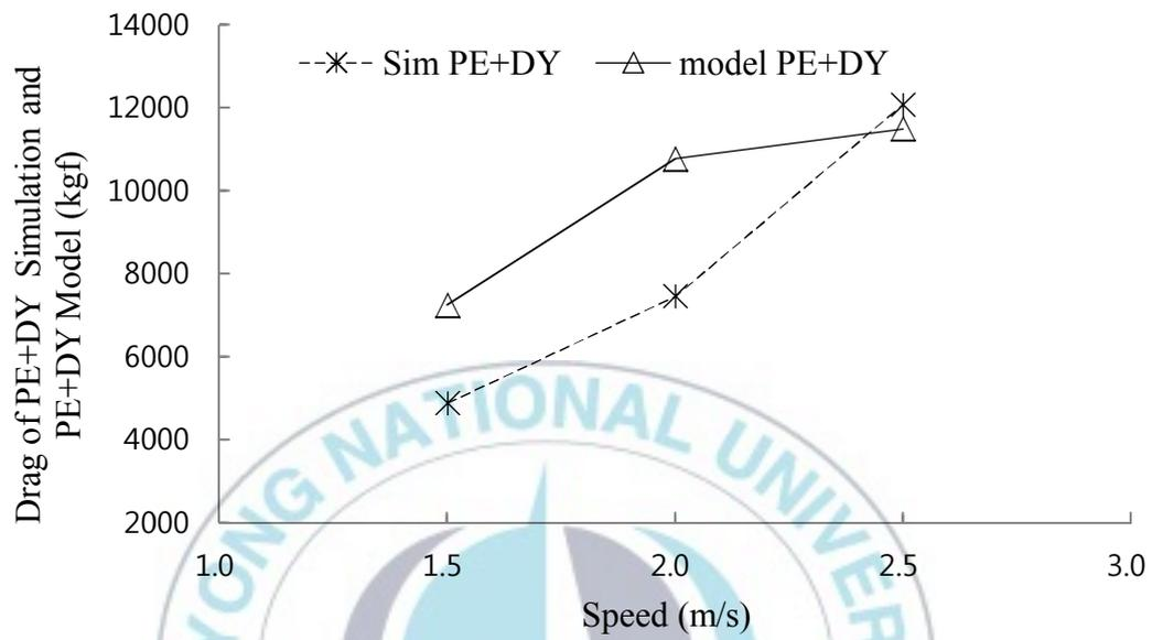
Fig. 21. Relationship between towing speed and drag of PE+DY simulation and PE+DY model.
