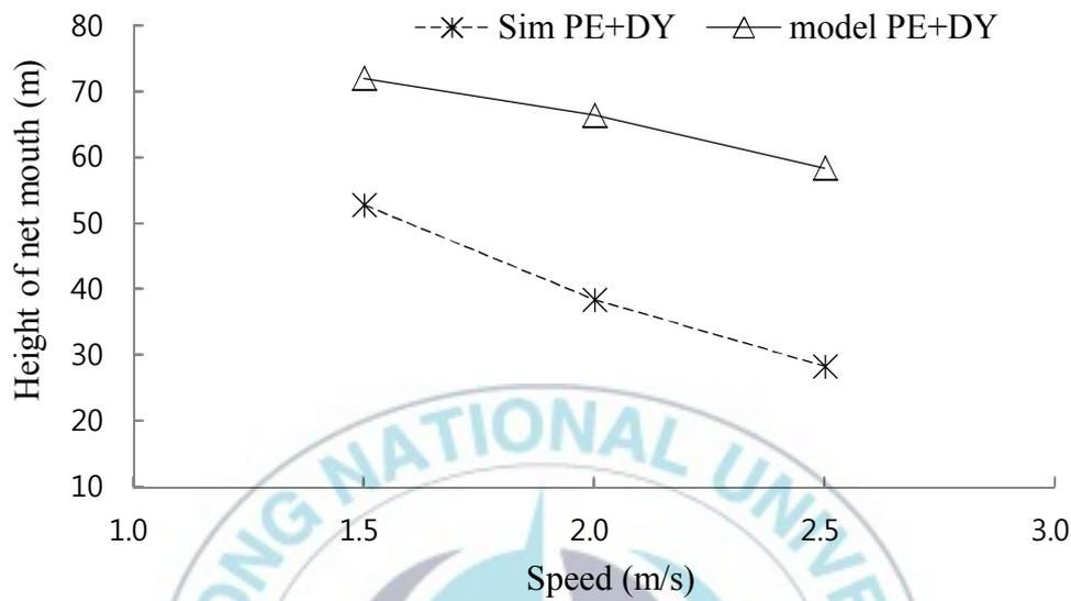
Fig. 19. Relationship between height of PE+DY simulation and PE+DY model and towing speed.
