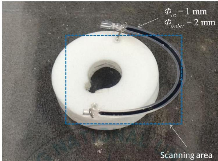
Fig. 5.4 Sample for PA imaging to use the PVDF transducer.
