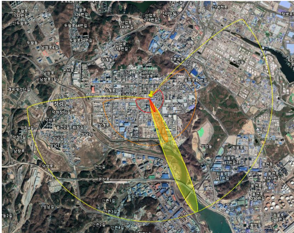
Fig. 10. Diffusion range mapping for 4inch hole release by Aloha (water curtain operating)
