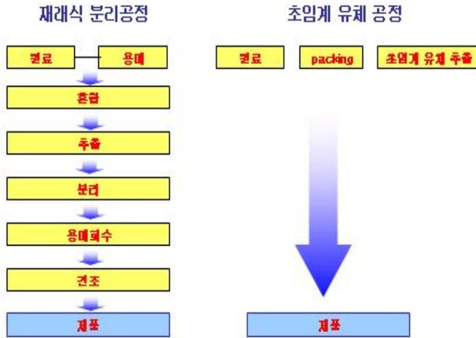
Fig. 4. Comparison of solvent extraction and SC-CO<sub>2</sub> extraction.
