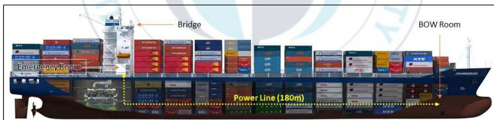
[Fig. 13] Ship-PLC+NMEA test bed and communication testing section
