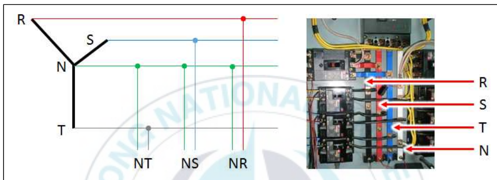
[Fig. 3] 3-phase 4-wire Y-connection (land-use power line structure)
