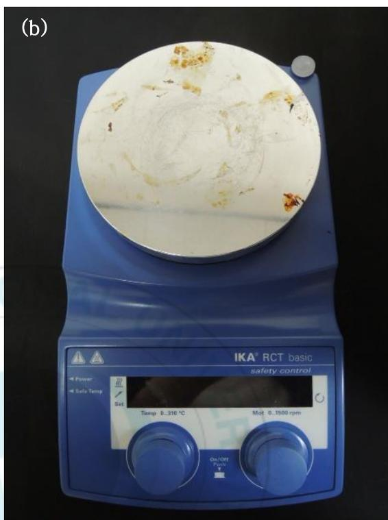
Figure 9. (a) Overhead stirrer (b) Hotplate & stirrer
