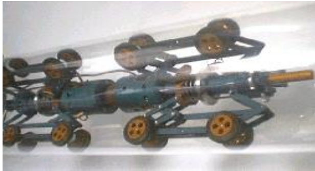
Fig. 1.5 Pipe inspection robot using tension spring
