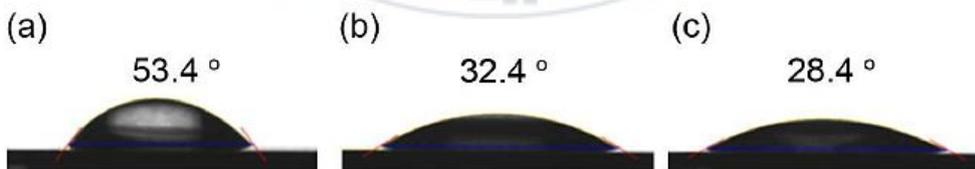
**Figure 2.7** Water contact angle images of (a) non-treated, (b) pDA-, and (c) pDA/TA-coated stainless steel surfaces.
