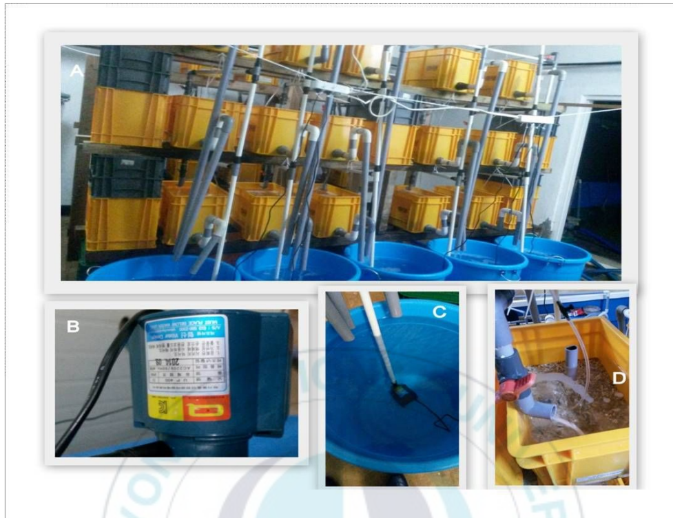
Fig. 6. Experiment set-up. (A) Arrangement of boxes and drums in the experiment room. (B) Pump. (C) Drum of water with pump. (D) Inside of box, showing inlet water and aerator.
