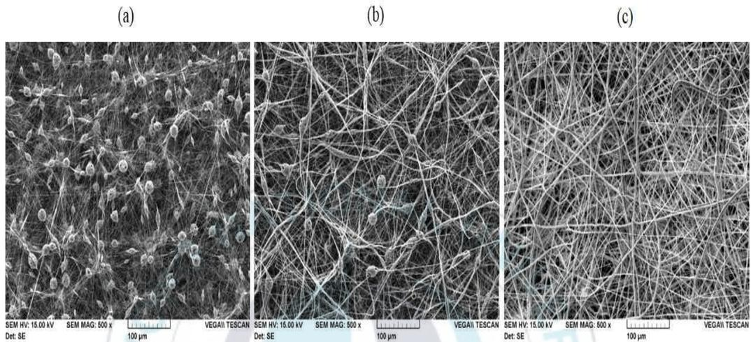
**Fig. 13.** SEM micrographs of electrospinning PCL fiber mats showing the morphology change at different PCL polymer concentration. (a) 8% PCL solution, (b) 10% PCL solution and (c) 12% PCL solution. Voltage = 7.2 kV, distance to collector = 15 cm.
