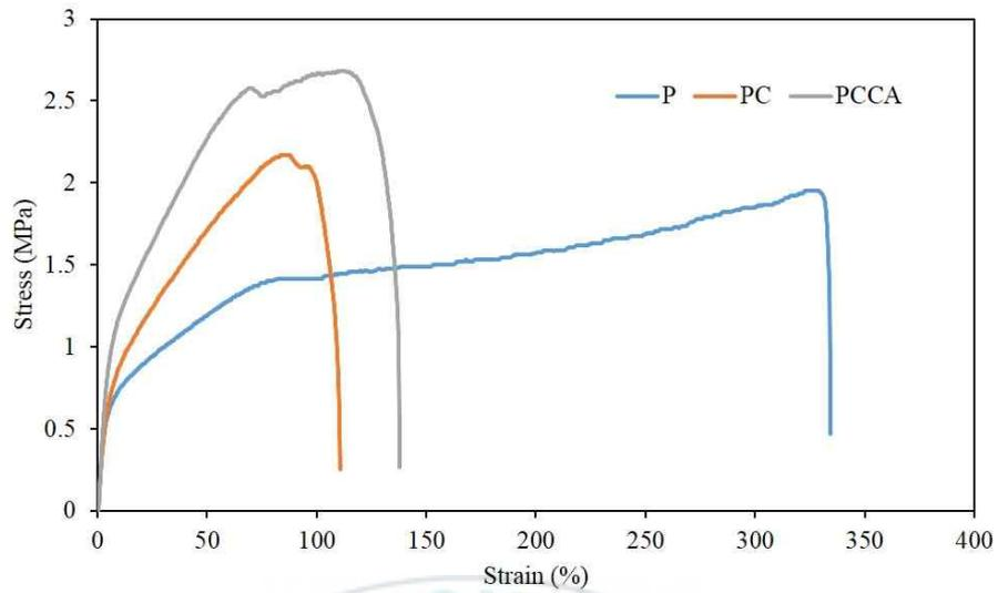
**Fig. 17.** Stress-strain curve of non-loaded PCL (P), chitosan-loaded PCL (PC) and chitosan-caffeic acid PCL (PCCA) nano/microfiber mats.
