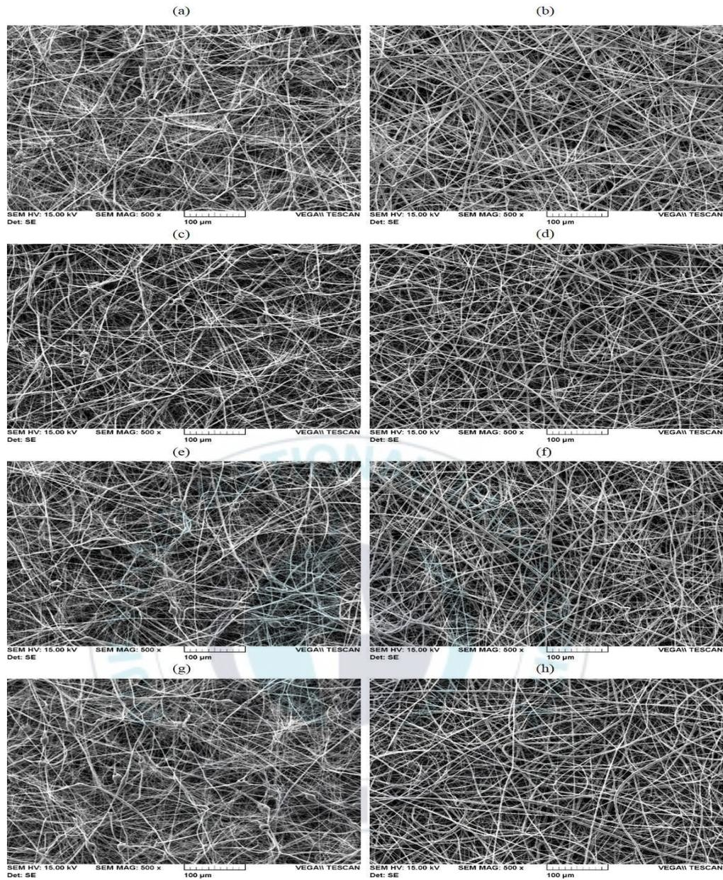
**Fig. 14.** SEM micrographs of electrospinning PCL polymer membrane showing the morphology change at different condition. 10% PCL solution (A, 18 cm, 8.5 kV; C, 21 cm, 9.6 kV; E, 24 cm, 10.5 kV; G, 27 cm, 11 kV) and 12% PCL solution (B, 18 cm, 8.5 kV; D, 21 cm, 9.6 kV; F, 24 cm, 10.5 kV; H, 27 cm, 11 kV)
