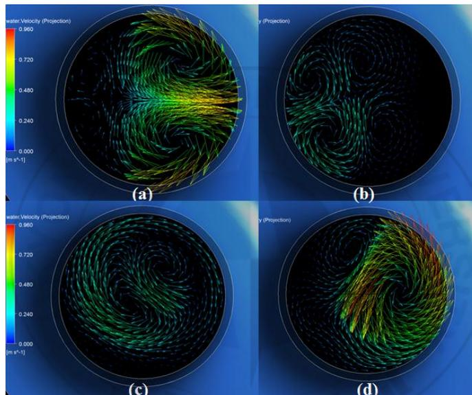
Fig 5.3 Velocity in pipe swirl meter.
