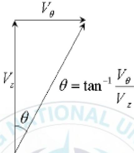
Fig. 2.5. Angle of velocity
