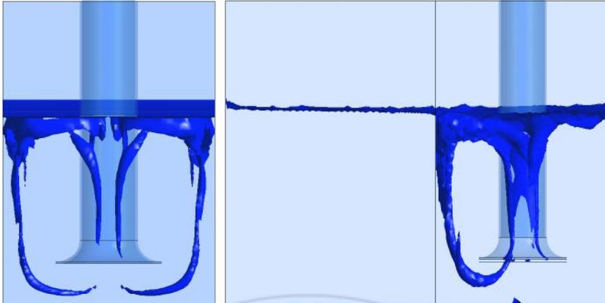
Fig 5.5. Line model-Front and L-Type model-Front view
