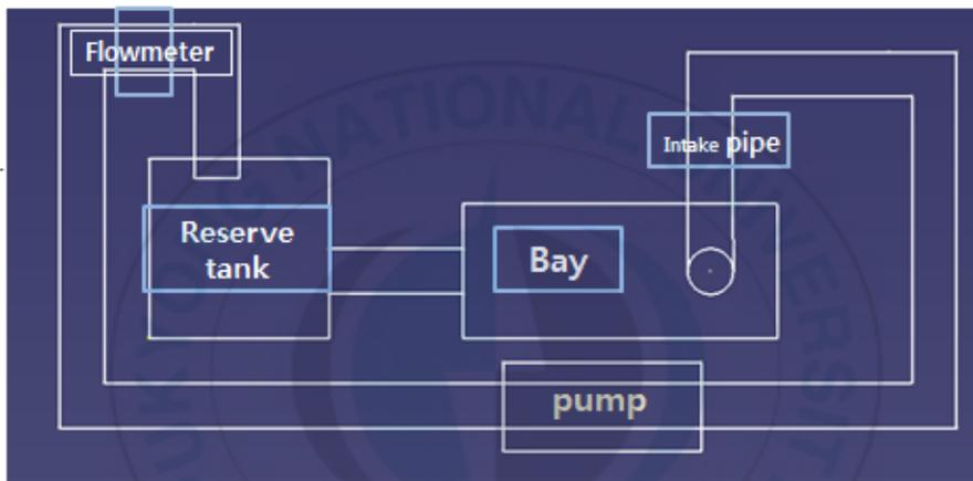
Fig. 2.2. Circulation system of pump sump
