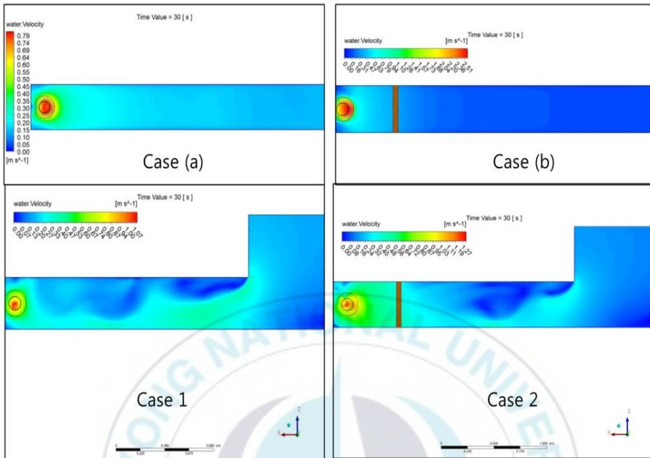
Fig 5.4 Comparing between the line case and L-Type case.
