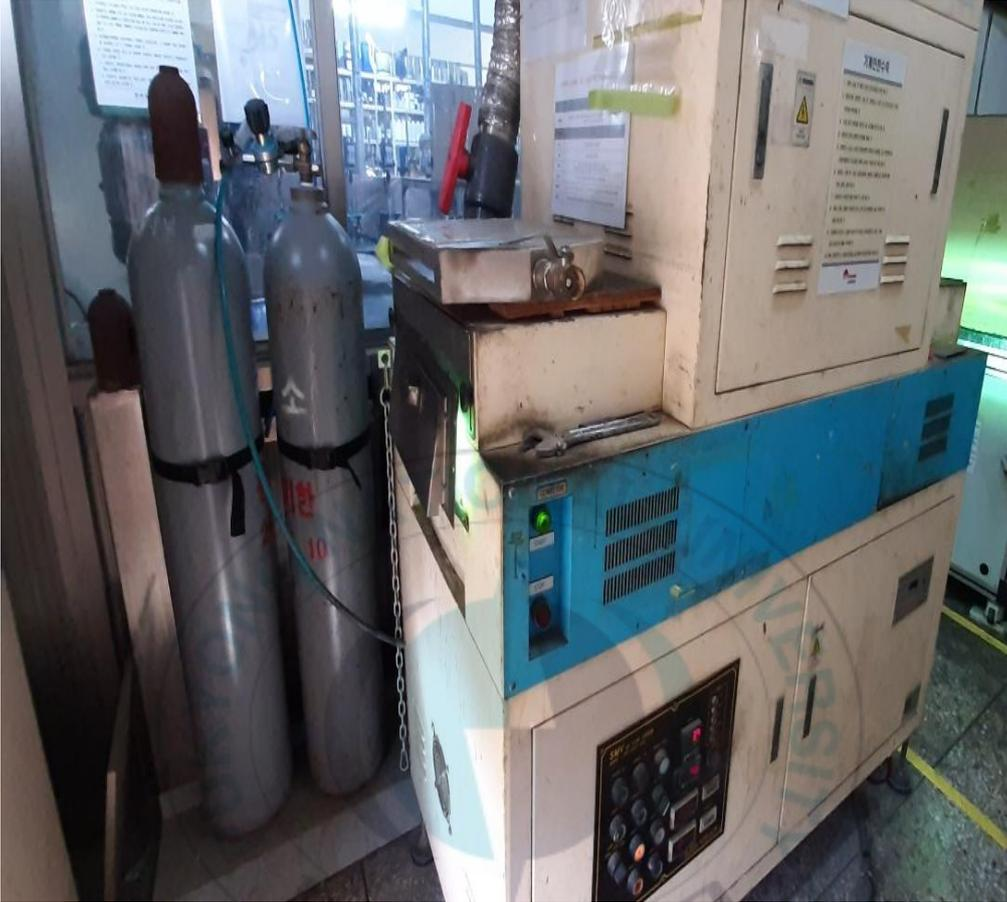
Figure 3.1. UV Curing system.
