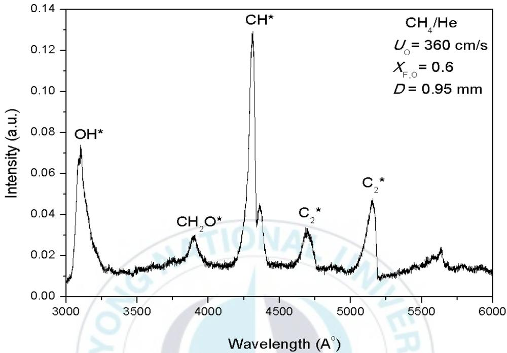
Fig. 9 Spectral wavelength scan of the lifted flame
