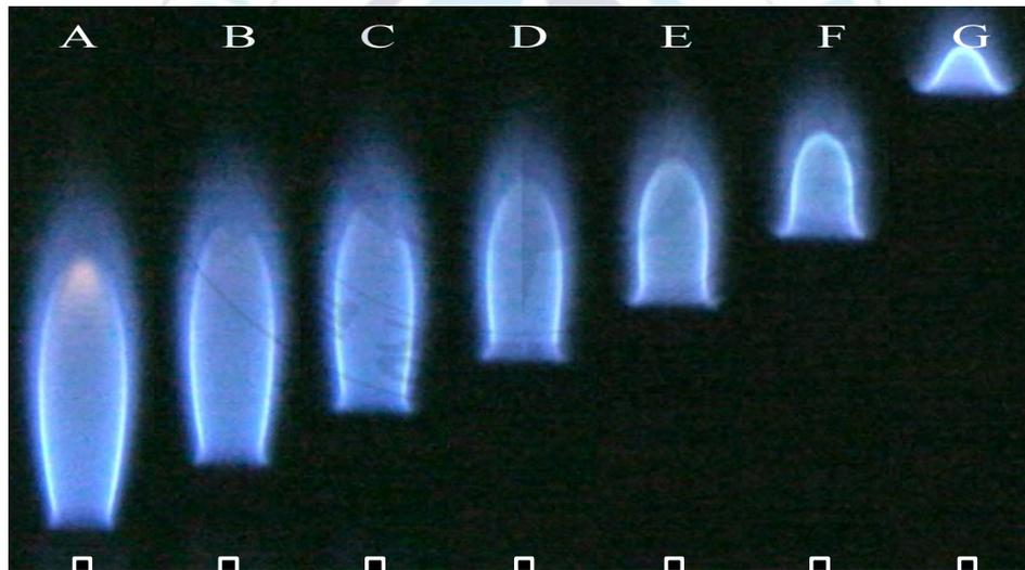
Fig. 3 (a) Change in liftoff height with fuel nozzle exit velocity for methane diluted with helium ( $Sc < 1$ ) at various  $X_{F,O}$  and (b) direct photographs of lifted methane jet flame diluted with helium for  $U_o = 260$  cm/s, at (A)  $X_{F,O} = 0.6$  (B) 0.56 (C) 0.52 (D) 0.48 (E) 0.44 (F) 0.4 (G) 0.36
