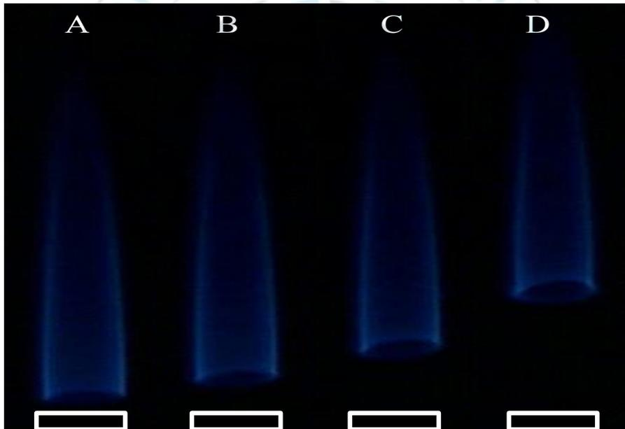
Fig. 6 (a) Change in liftoff height with fuel nozzle exit velocity for methane diluted with nitrogen ( $Sc < 1$ ) at various fuel mole fractions and (b) direct photographs of stationary lifted methane jet flame diluted with nitrogen for  $U_o = 20$  cm/s at (A)  $X_{F,O} = 0.32$  (B) 0.31 (C) 0.3 (D) 0.29.
