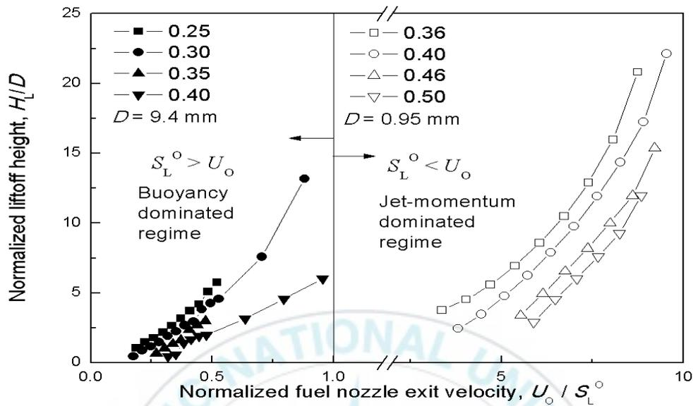
Fig. 4 Normalized liftoff height with fuel nozzle exit velocity considering stoichiometric un-stretched non-adiabatic laminar burning velocity for two different fuel nozzles.
