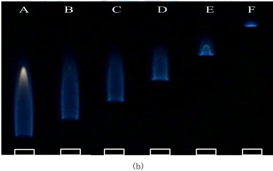
Fig. 2 (a) Change in liftoff height with fuel nozzle exit velocity for methane diluted with helium ( $Sc < 1$ ) at various  $X_{F,O}$  (b) direct photographs of stationary lifted methane jet flame diluted with helium for  $U_o = 14$  cm/s, at (A)  $X_{F,O} = 0.45$  (B) 0.4 (C) 0.35 (D) 0.3 (E) 0.25 (F) 0.22.
