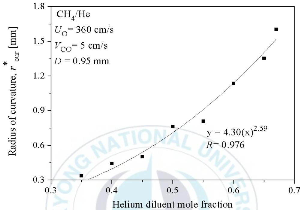
Fig. 11 Radius of curvature  $r_{\text{cur}}^*$ , of lifted methane jet flame with the addition of helium dilution by using 0.95 mm nozzle diameter.
