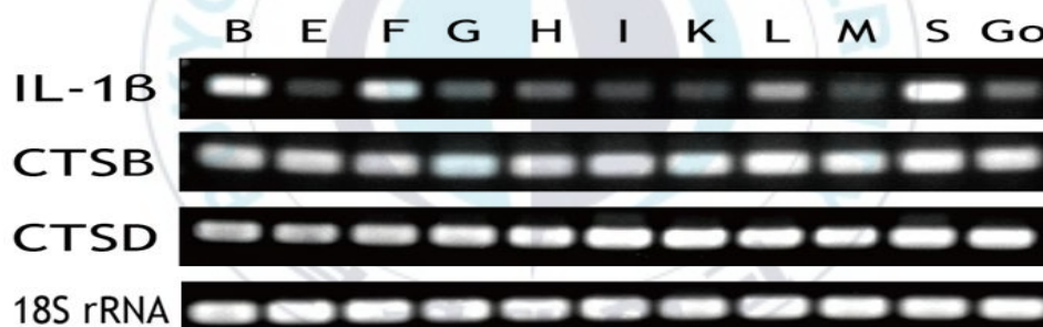
Figure 12. RT-PCR analysis of Siberian sturgeon IL-1 \beta , CTSB and CTSD gene mRNA expression in tissues. Such as Brain (B), Eye (E), Fin (F), Gill (G), Heart (H), Intestine (I), Kidney (K), Liver (L), Muscle (M), Spleen (S) and Gonad (Go). Confirmed by 1.5% agarose gel electrophoresis.
