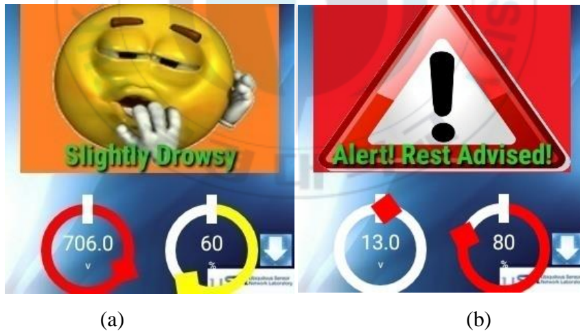
Figure 6.6: (a) slightly drowsy interface with 1Hz vibration, (b) serious drowsy detected with 2 Hz vibration activated.
