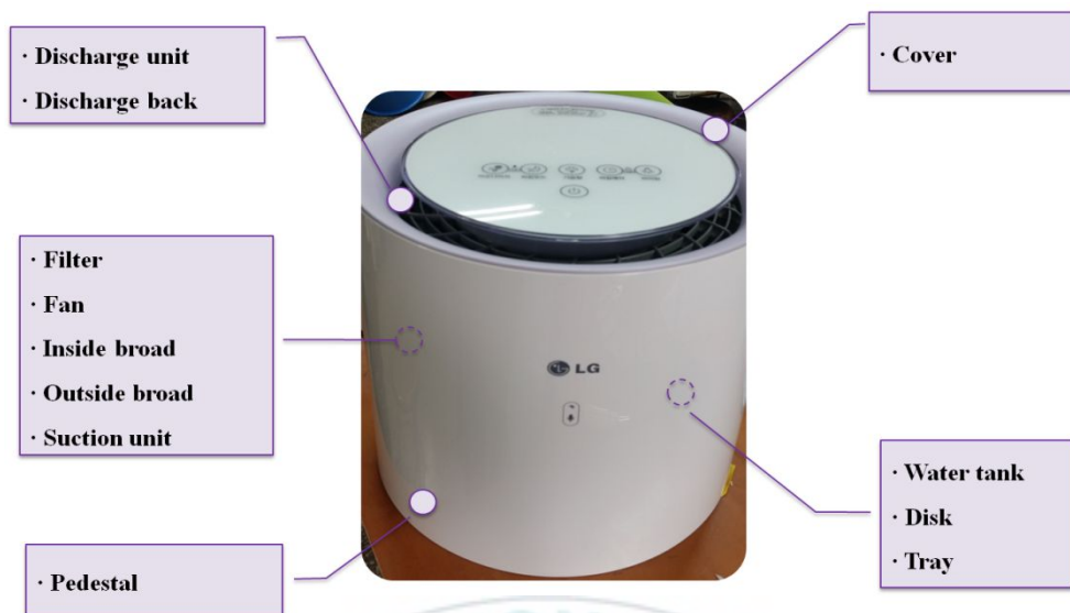
Fig. 5. Sample collection parts using swab test in product A.
