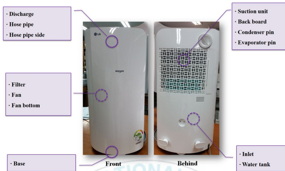
Fig. 8. Sample collection parts using swab test in product D.
