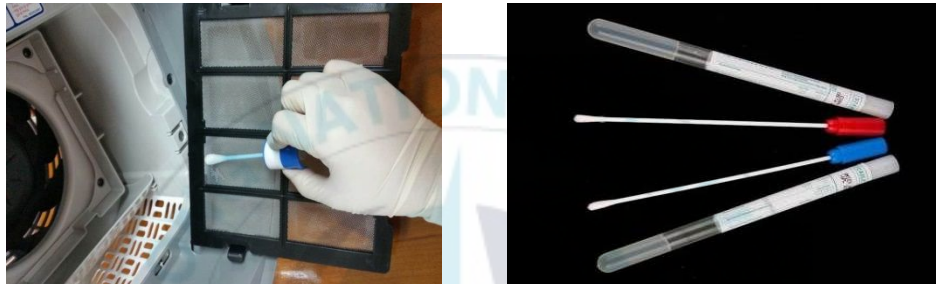
Fig. 2. Sample collection using swab test from air solution products.
