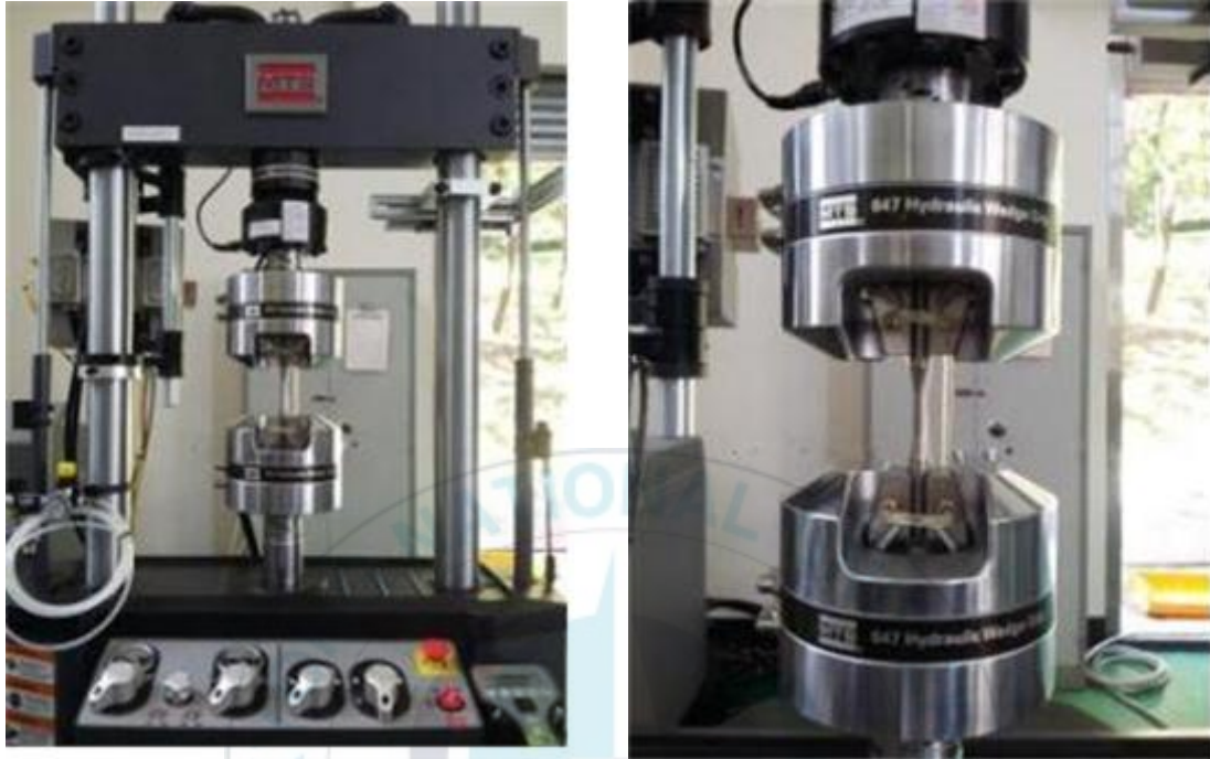
Fig. 14 Photos of the specimen set-up(100kN MTS Landmark, Model 370)
