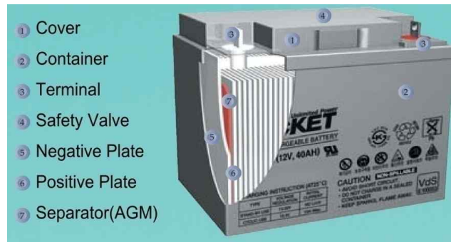
Fig. 3.12 Structure of Battery
