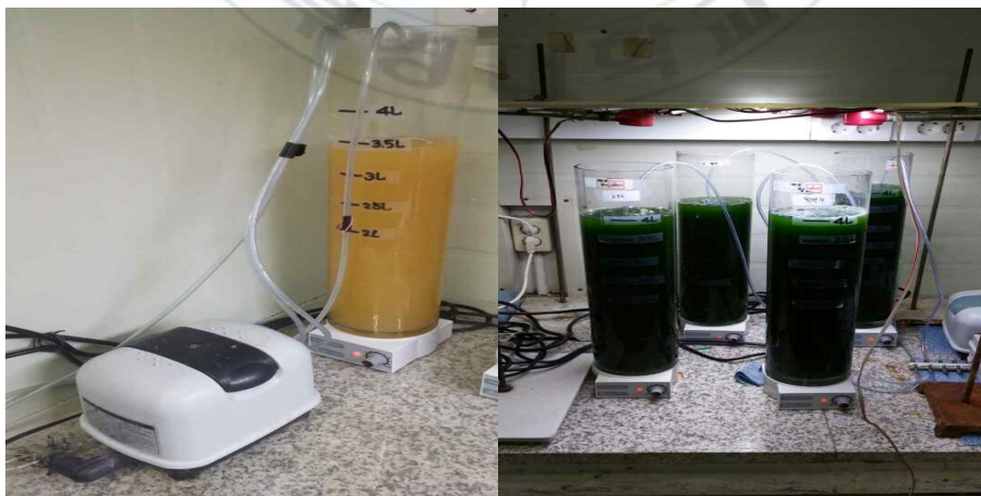
Fig. 3.1 Operation of activated sludge reactor and algae culture reactor
