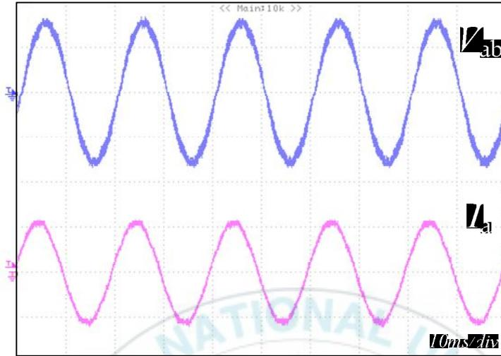
(a)  $P = 3 \text{ [kW]}, V_{DC} = 350 \text{ [V]}, V_{ab} = 220 \text{ [V]}, I_a = 7.87 \text{ [A]}$
