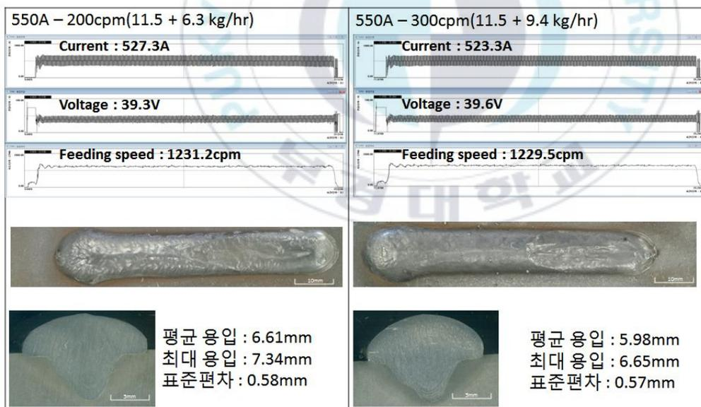
Table 4.8 Waveform, Bead appearance & Cross section
