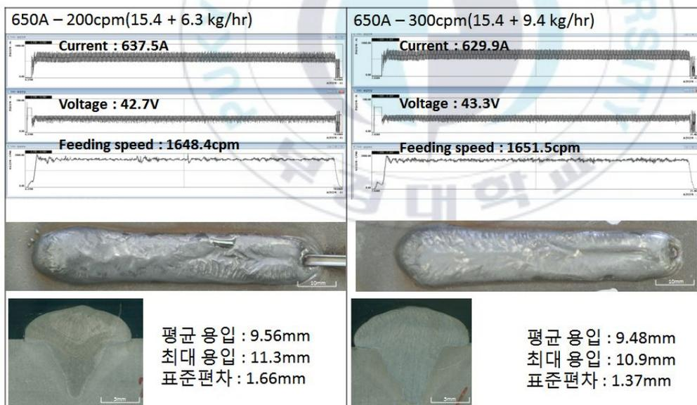
Table 4.12 Waveform, Bead appearance & Cross section
