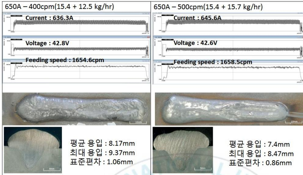
Table 4.13 Waveform, Bead appearance & Cross section
