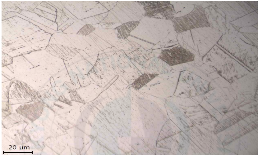
Fig. 1 Optical micrograph of 202 austenitic stainless steel
