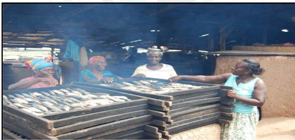
<Figure 6> Fish packed on tier of chorkor trays for smoking
