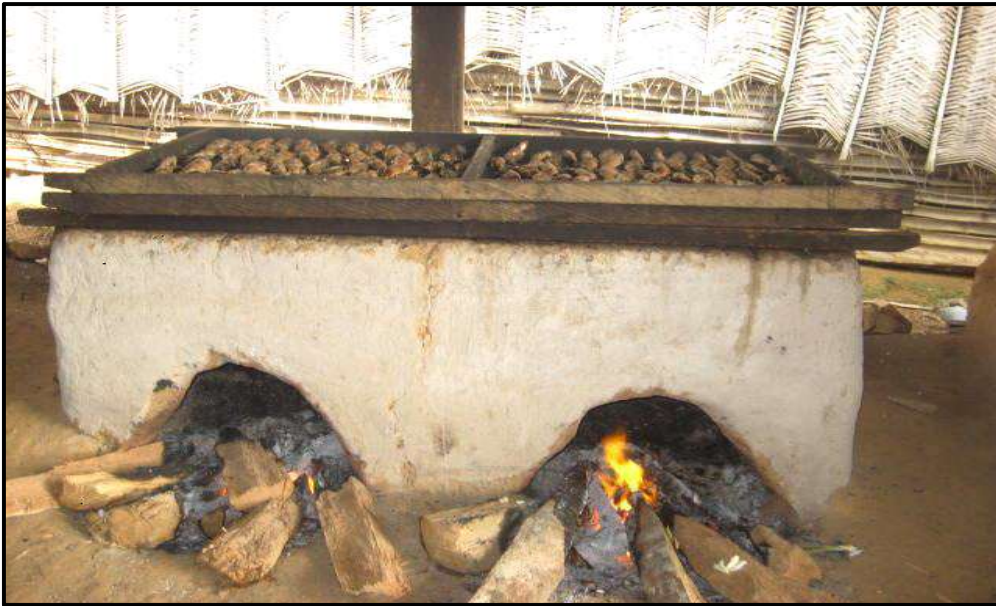
<Figure 4> Chorkor smoked oven with fish on tier trays for smoking
