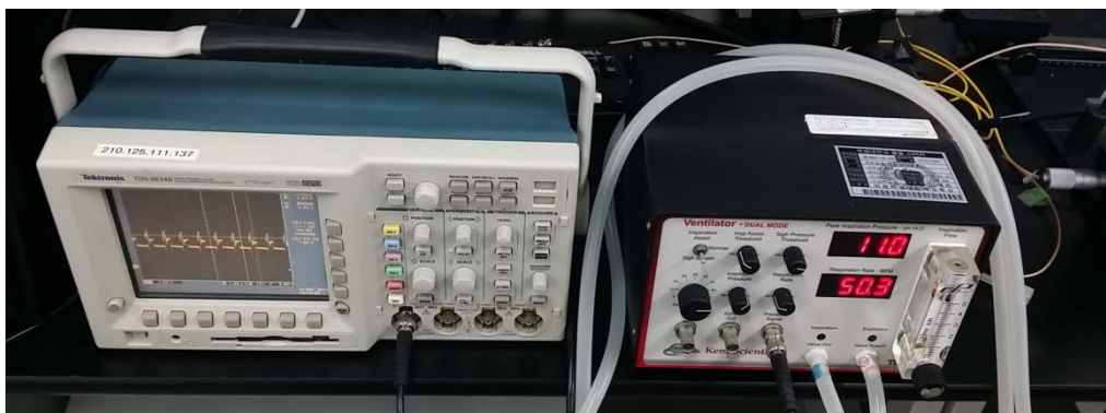
Figure II.18 The ventilator can check the respiratory waveform with connecting an oscilloscope by BNC cable.
