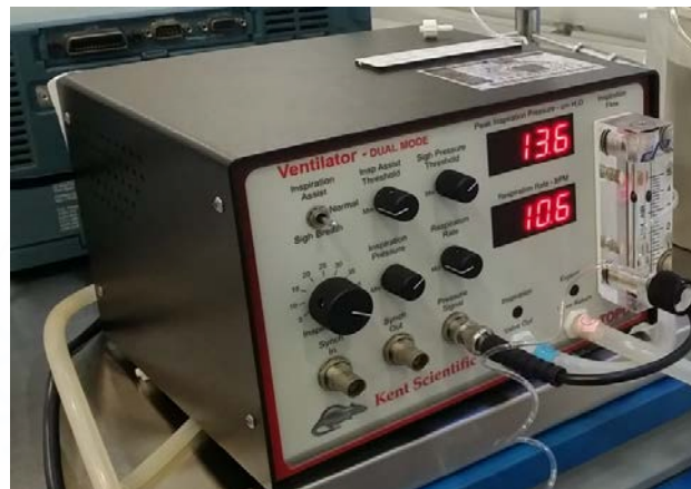
Figure II.17 Ventilator TOPO (Kent Scientific) for animals.
