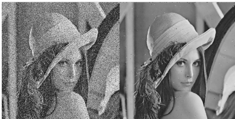
Figure 4. Example of an image with ‘salt and pepper’ noise and its result after median filtering
