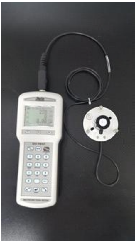
Figure 4. DeltaLogger DO9847 and illuminance sensor LP471HPHOT
