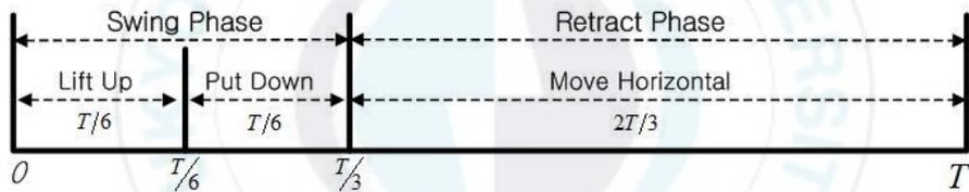
Fig. 4.6 Each state time in one cycle time of the quadruped gait
